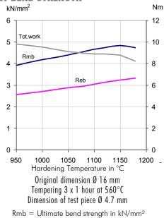
Rmb = Ultimate bend strength in kN/mm<sup>2</sup> Reb = Bend yield strength in kN/mm<sup>2</sup> Tot. work = Total work in Nm
